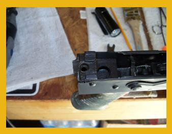
Now using a bench grinder, you need to grind the stub flush for proper fit of the Stock Receiver Block. I removed the pistol grip so it's easier to grip and handle while grinding the tang stub
